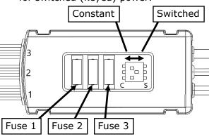
The output leads have two wires: the red wire is positive, and the black wire is negative. Two options are provided for wiring outputs: Three Pigtails or Three Connectors with 2.8mm Terminals.
